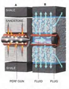
PLUG AND PERFORATION A plug blocks off a section of pipe, and a "perf gun" blasts small holes in the sandstone (A). Fluid is pumped in at high pressure (B), releasing the oil. SLIDING SLEEVE Plastic balls are forced down the pipe, pushing open sliding sleeves to expose holes in the pipe. Fluid shoots out through the holes, fracturing the rock.
